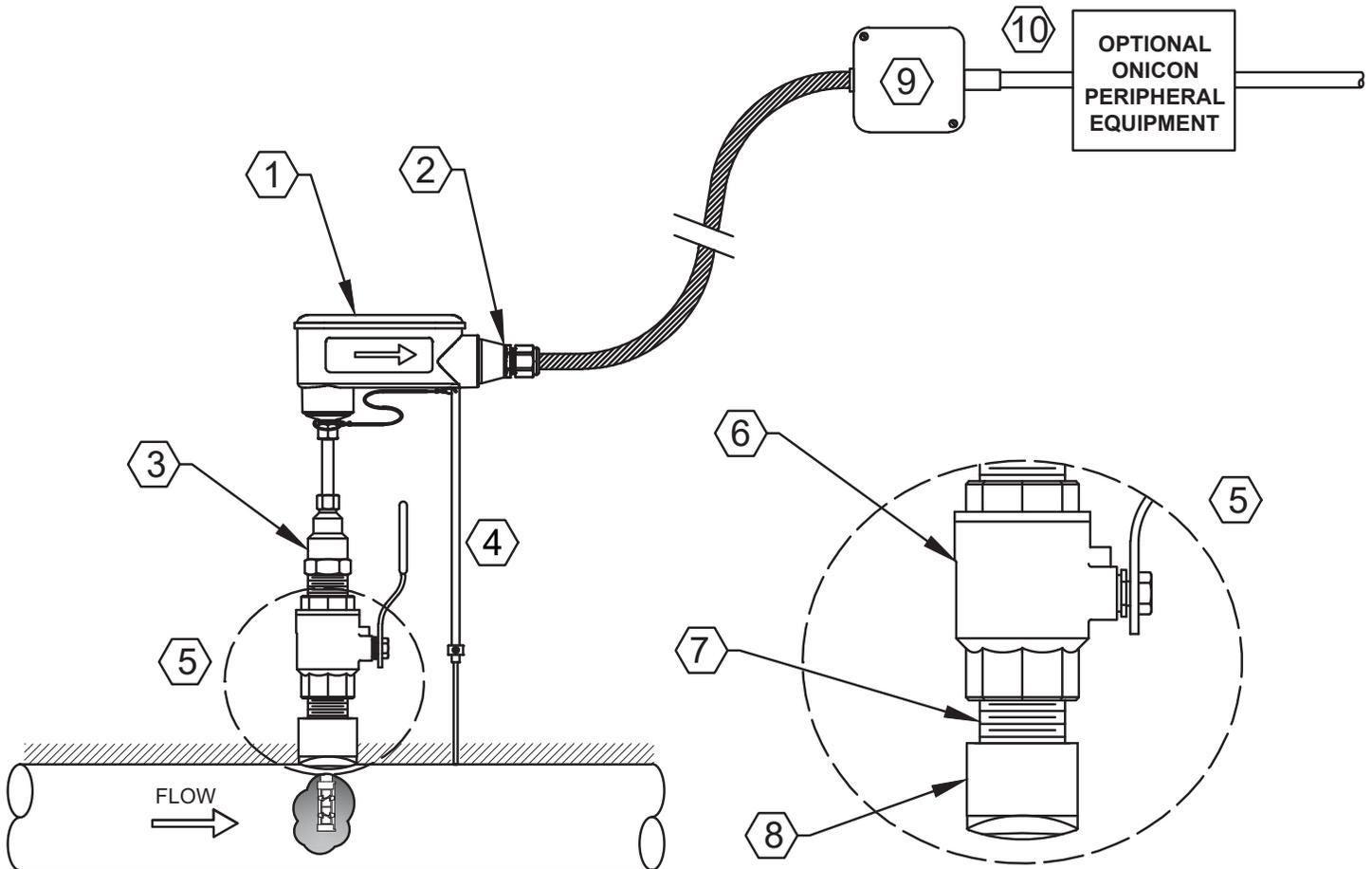
1. Electronics enclosure with flow direction indicator
