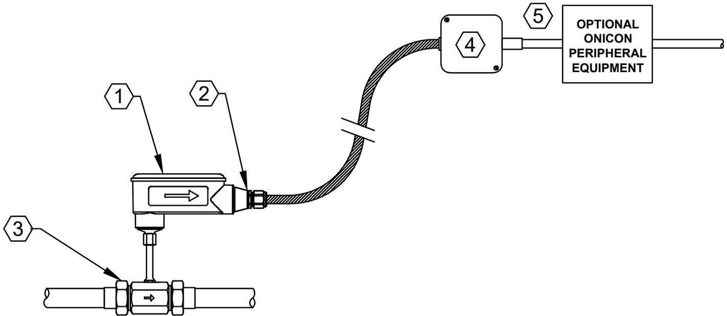
1. Electronics enclosure with flow direction indicator
