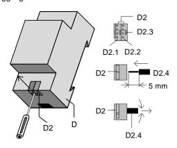
Figure 4: Connecting / disconnecting bus cables
