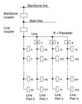
Figure 1. Connection of repeaters to a bus line
