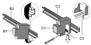
Figure 3: Mounting / dismounting a DIN-rail device
