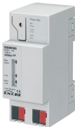
The line-/ backbone coupler provides a data connection between two separate KNX bus lines and isolates the bus lines from each other to enable the independent local operation of a bus line.
