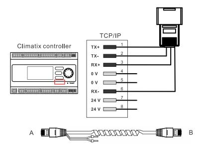
**Note:** Don't mix up RS485 connection with TCP/IP connection. The maximum cable length supported is 100 m.
