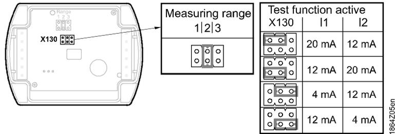
The setting element is located inside the cover. It comprises 6 pins and a jumper. It is used to select the required measuring range and to activate the test function.
