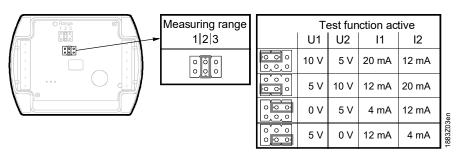
The setting element is located inside the cover. It consists of 6 pins and a shorting plug. It is used for selecting the required temperature measuring range and for activating the test function.
