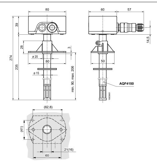
Drilling template with (without) mounting flange
