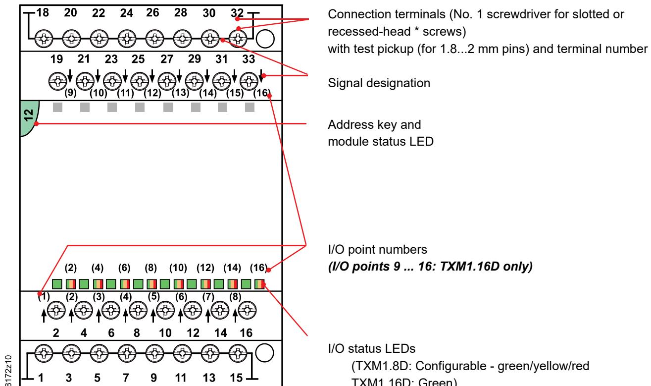
Connection terminals (No. 1 screwdriver for slotted or recessed-head \* screws)
