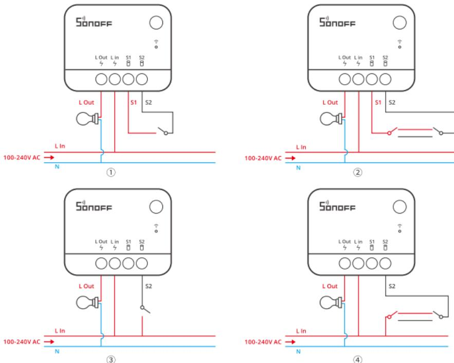
**⚠ For the above ③④ wiring methods, please ensure the proper wiring and powering of the L In terminal, otherwise it will cause the device to work abnormally.**
