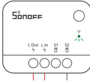
After powering on, the device will enter the pairing mode defaulted during the first use and the green LED indicator will "flash slowly".
